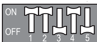
Figure 127: LMU481-541-601HV Saving Power Consumption with Mode Lock DIP Switch Settings.
