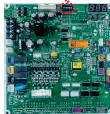
Figure 118: LMU180-240HV-30-36CHV Forced Cooling DIP Switch Setting.
